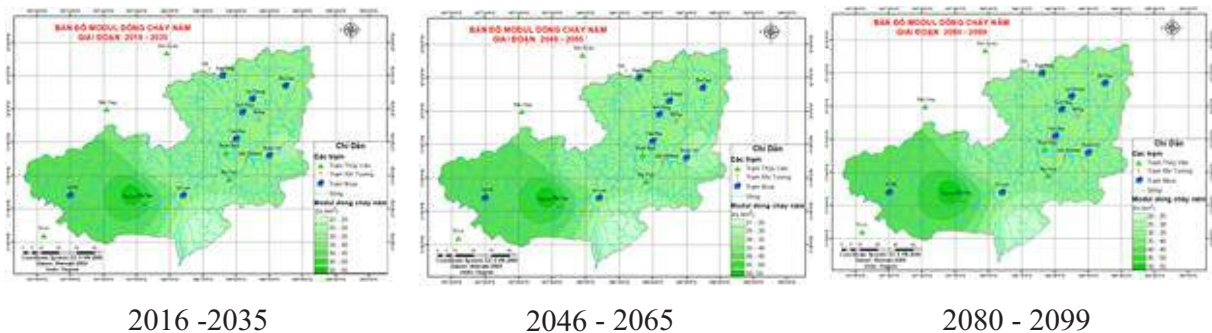
Fig. 8. River basin flow module according to RCP scenario 4.5 (l/s.km 2 )
